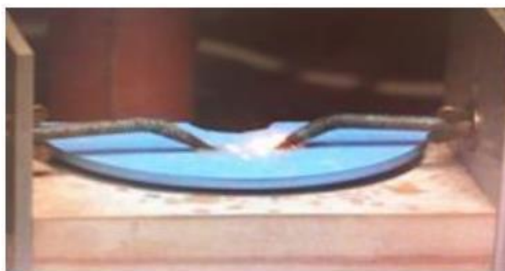
Fig.1 Flashover on silicone rubber specimen
